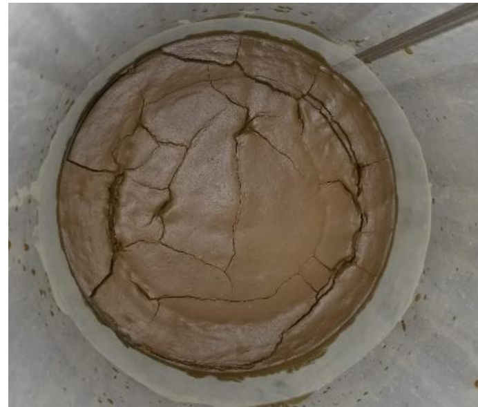
Filtration of Ni, Mn, Co Hydroxide in Air
